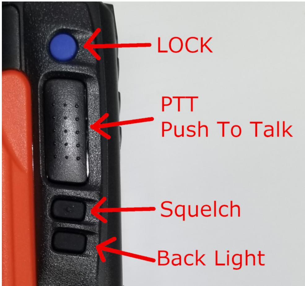
Press the squelch button and while holding this button down rotate the volume knob clockwise for more volume or counter-clockwise for less volume.
