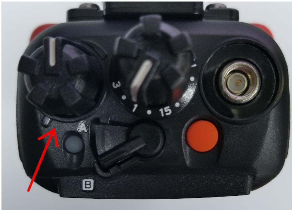
In this image the red arrow is pointing at the power switch. The switch is on as indicated by the white line pointing at the back of the radio. NOTE: In order to get a good photo of the top of the radio the antenna has been removed. **Your radio should always have an antenna attached before turning the radio on!**
