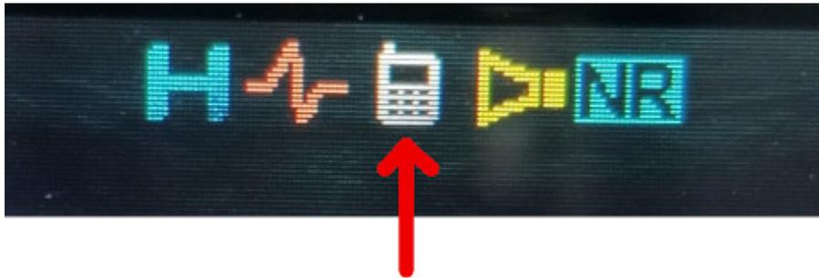
You **do not** want to have the radio in this mode. After you have set the correct zone and channel and locked the keypad check the display to make sure this icon is **not** shown. If it does appear, unlock the keypad (blue button) and press the "A" key one time to disable "talk around" mode. Then lock the keypad again.
