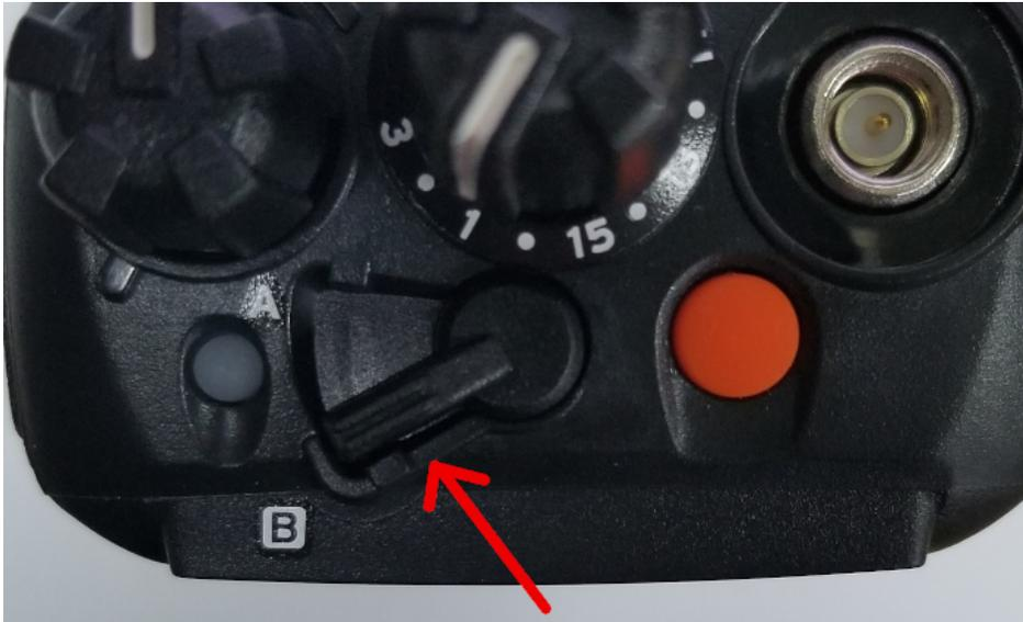
Setting "A" is high power. Setting "B" is low power. The front panel icons will show "H" or "L" to indicate the power level. The letter "H" will be displayed in blue when in high power. The letter "L" will be displayed in yellow when in low power.
