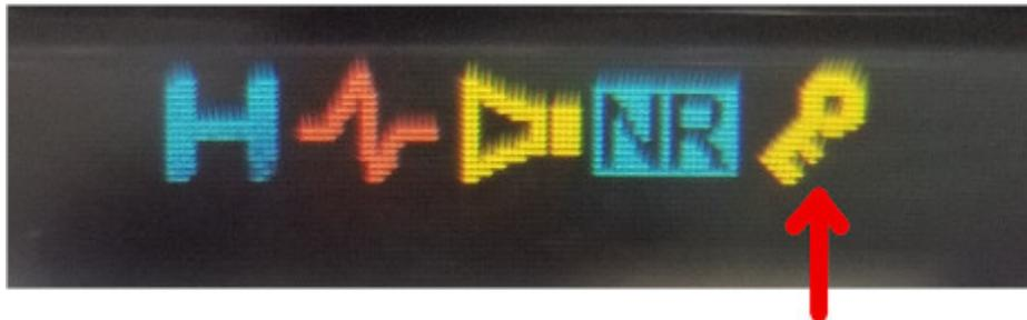
**For normal use set the radio to the desired zone and then lock the keypad.** This will prevent accidentally touching a button on the keypad and changing a setting.
