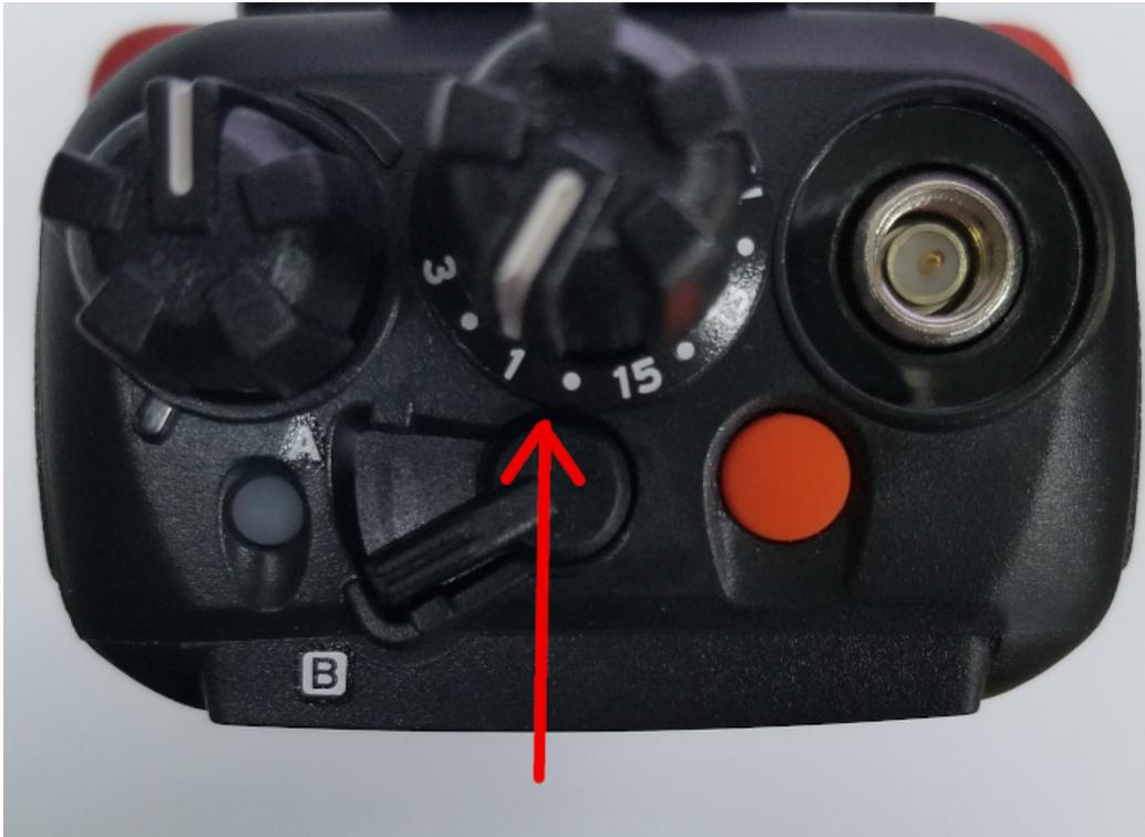
Rotate the channel knob counter clockwise so the white line is pointing to the number 1. This sets the radio to channel 1 which is "MRC Command", the Cannon Beach MRC repeater.
