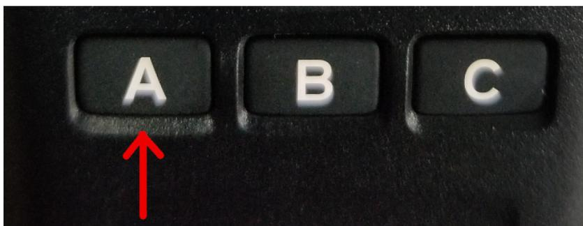
Press the "A" key several times while watching the icons displayed above the text on the screen. A small white symbol of a radio indicates that the radio is in "talk around" mode.
